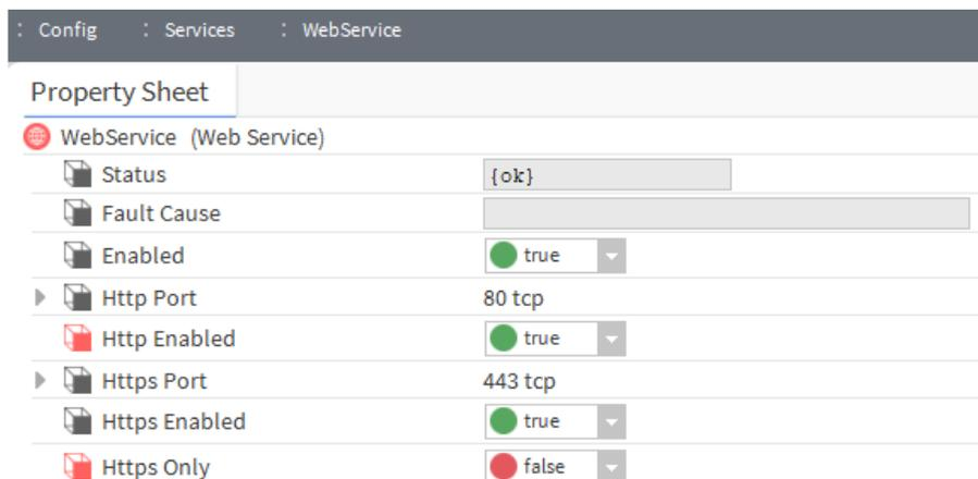
Figure 42. Proper WebService configuration for HDMI support
