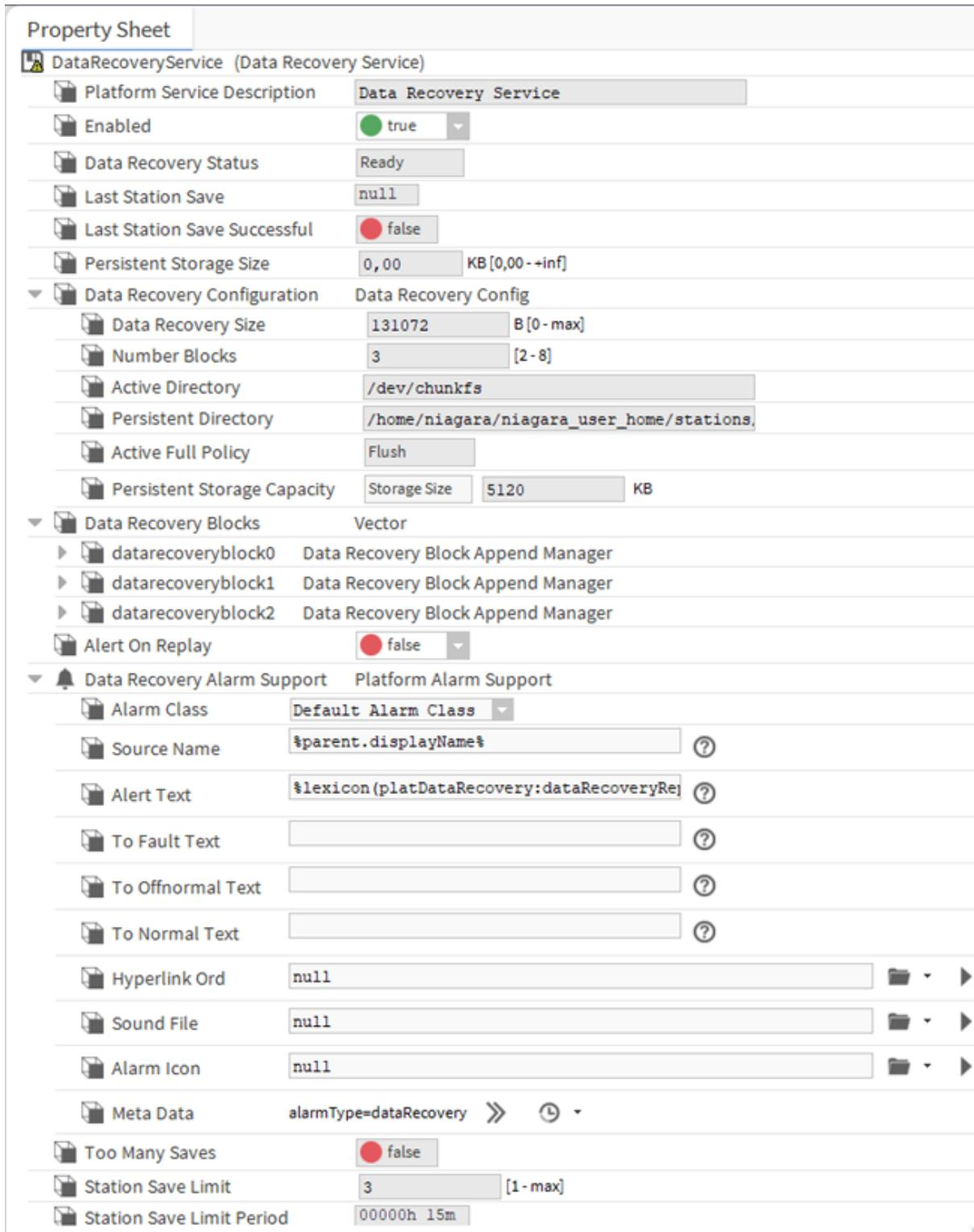
Figure 36. MAC36 Platform Service Properties view of DataRecoveryService
