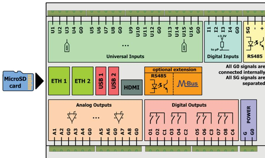
Figure 3. Block diagram
