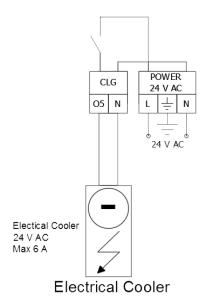
Figure 21 Digital Output 05, an example of 24 V AC Electrical Cooler connection (iSMA-B-FCU-LL version)
