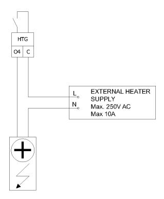
Figure 19 Digital Output 04, exemplary Electrical Heater connection
