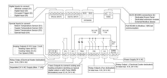
Figure 4 iSAM-B-FCU-LL diagram of terminals and internal connections
