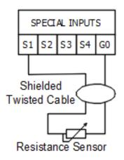
Figure 14 Connection of Special Inputs resistance sensor
