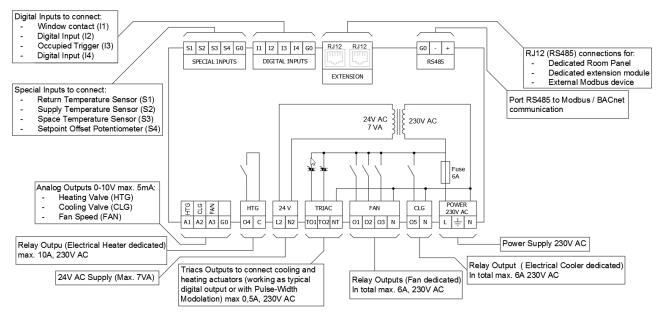
Figure 2 iSMA-B-FCU-HH diagram of terminals and internal connections
