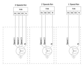
Figure 18 Digital Outputs 01-03, example of fan connections
