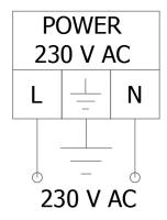
Figure 5 230 V AC Power supply connection
