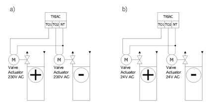
Figure 17 Connection between Thermal Valves and Triac Outputs: a) iSMA-B-FCU-HH; b) iSMA-B-FCU-HL, and iSMA-B-FCU-LL
