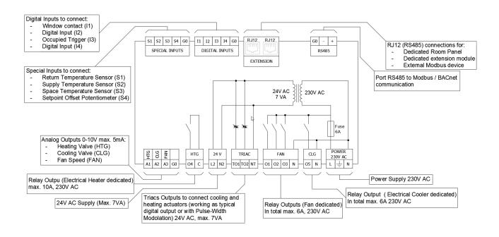
Figure 3 iSMA-B-FCU-HL diagram of terminals and internal connections
