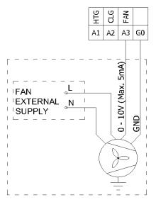
Figure 23 Analog Outputs, an exemplary connection of analog 0-10 V fan control
