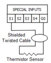
Figure 15 Connection of Special Inputs NTC sensor
