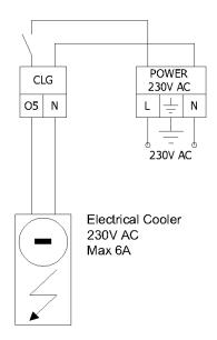
Figure 20 Digital Output 05, an example of 230 V AC Electrical Cooler connection (iSMA-B-FCU-HH and iSMA-B-FCU-HL version)
