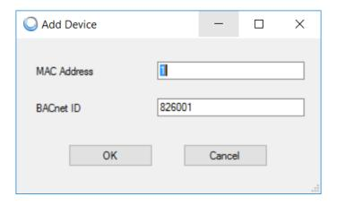
Figure 21 - Manually adding a device on BACnet
