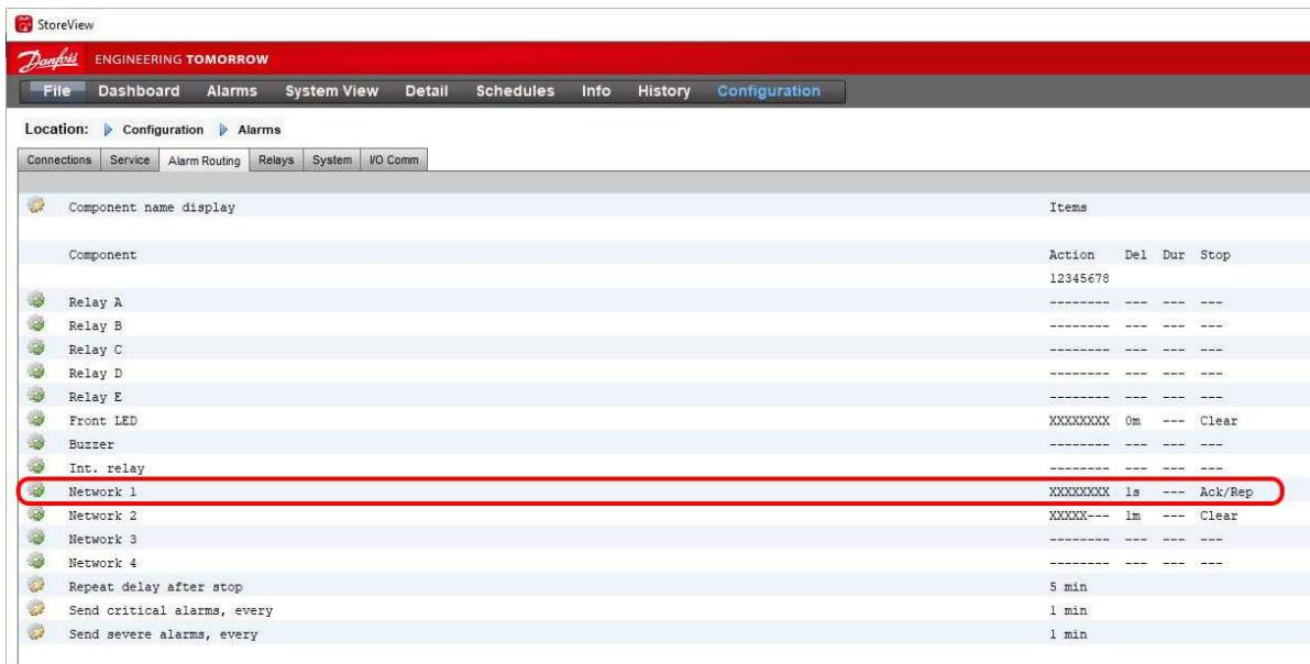
The screenshot shows the 'Alarm Routing' section of the configuration interface. A red box highlights the 'Network 1' entry in the list of components. Other entries include 'Component name display', 'Component', 'Relay A', 'Relay B', 'Relay C', 'Relay D', 'Relay E', 'Front LED', 'Buzzer', 'Int. relay', 'Network 2', 'Network 3', 'Network 4', 'Repeat delay after stop', 'Send critical alarms, every', and 'Send severe alarms, every'. Each entry has columns for 'Action', 'Del', 'Dur', and 'Stop'.
