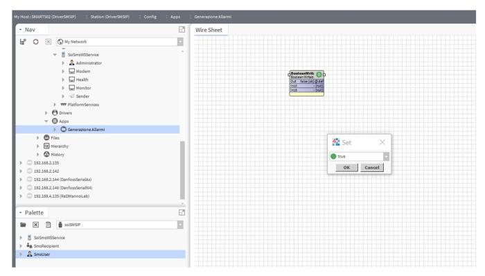
In its Wire Sheet, create a Boolean Writable point with a Boolean Chang Of State Alarm Extension, as shown in the following figure:
