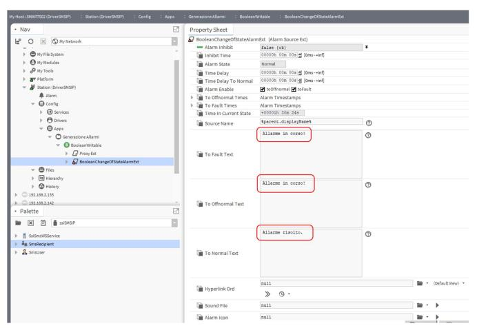
In the Property Sheet of the Alarm Extension, it is possible to specify the messages that will be generated and sent when the alarm occurs. All the other fields are according to Tridium standard rules.
