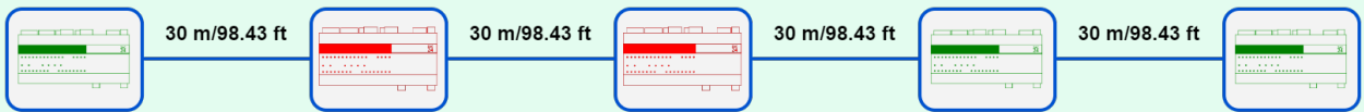
Total length of 90 m/295.28 ft between 2 working controllers and 30 m/98.43 ft to the next working controller - at no point does the distance between 2 working controllers exceed 100 m/328.08 ft
