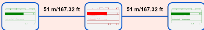
Total length of 102 m/334.65 ft between 2 working controllers exceeds the maximum range of 100 m/328.08 ft
