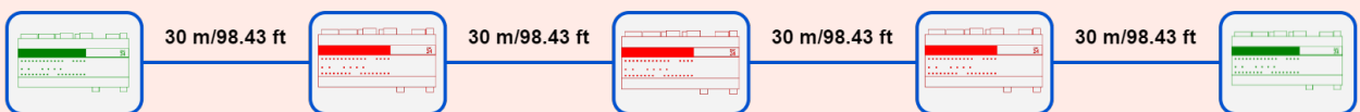
Total length of 120 m/393.7 ft between 2 working controllers exceeds the maximum range of 100 m/328.08 ft
